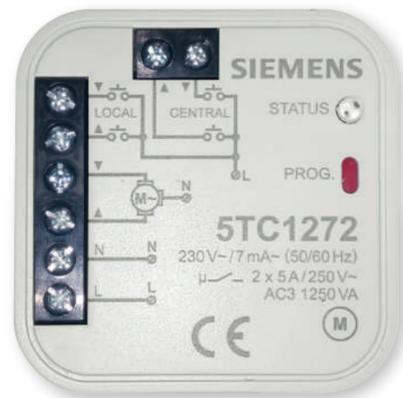
The 5TC1272 flush-mounted roller blind controller is used for local and/or central control of window roller blinds or other devices with single-phase 230VAC motors.
