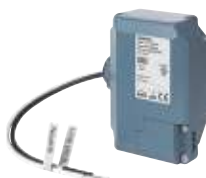
Distributed power supply 80mA 5WG1125-4CB23 Type: JB 125C23 Indoor mounting or attached to UL/NEMA Type connection boxes using a 1/2" threaded connector. 120 VAC 50..60 Hz power supply voltage.
