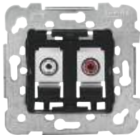
Stereo RCA socket outlet 18576 Rear screw-less terminal Cable: maximum 3 pairs of 0.3 mm 2
